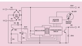
Schematic diagram - XP95 Optical Smoke Detector
